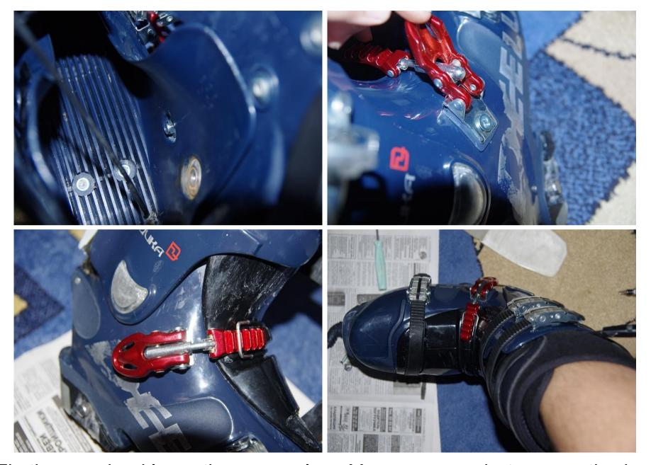
Fix the new buckle on the same place. You can use whatever method you like. I used a srew M6, 12 mm lenght of threaded part and nut with plastic clamp. Put a washer between a nut and boot shell and tighten well. That's all.
