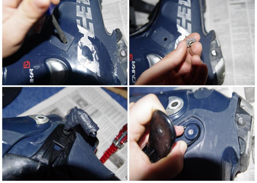
Knock out the rest of the clinch by something :-) I used a screwdriver. Remove plastic cover using deeluxe hex key and remove old or broken strap. Put new strap in the groove carefully and put plastic cover back. Tighten the bolt that fixes plastic cover.
