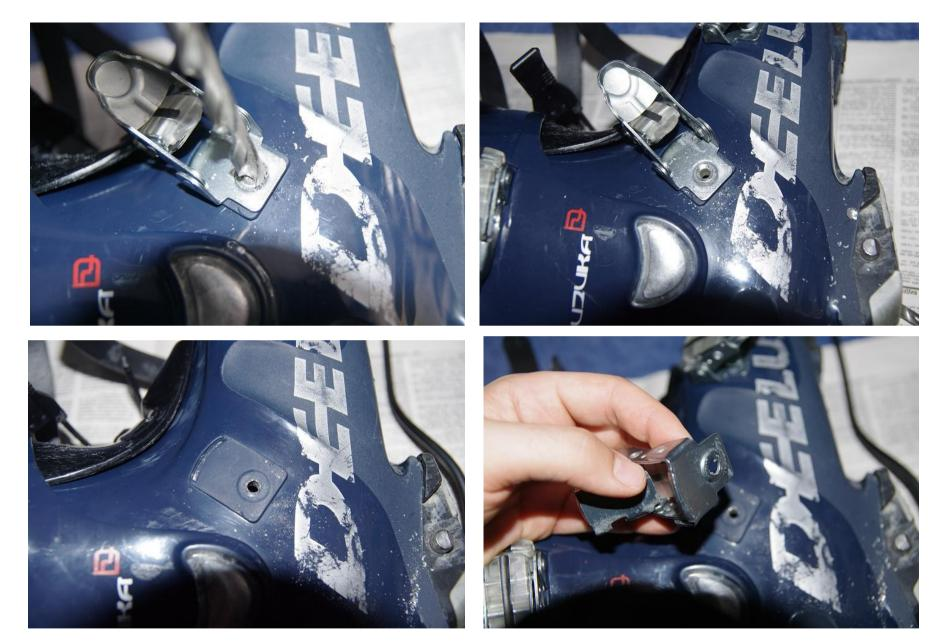
First we drill the head of the clinch by thicker drill . While drilling press drilling machine gently. Then use thin drill to remove the head completely. Do this carefully to avoid plastic shell damage.
